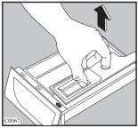
Remove the drawer by pressing the catch downwards and by pulling it out.
